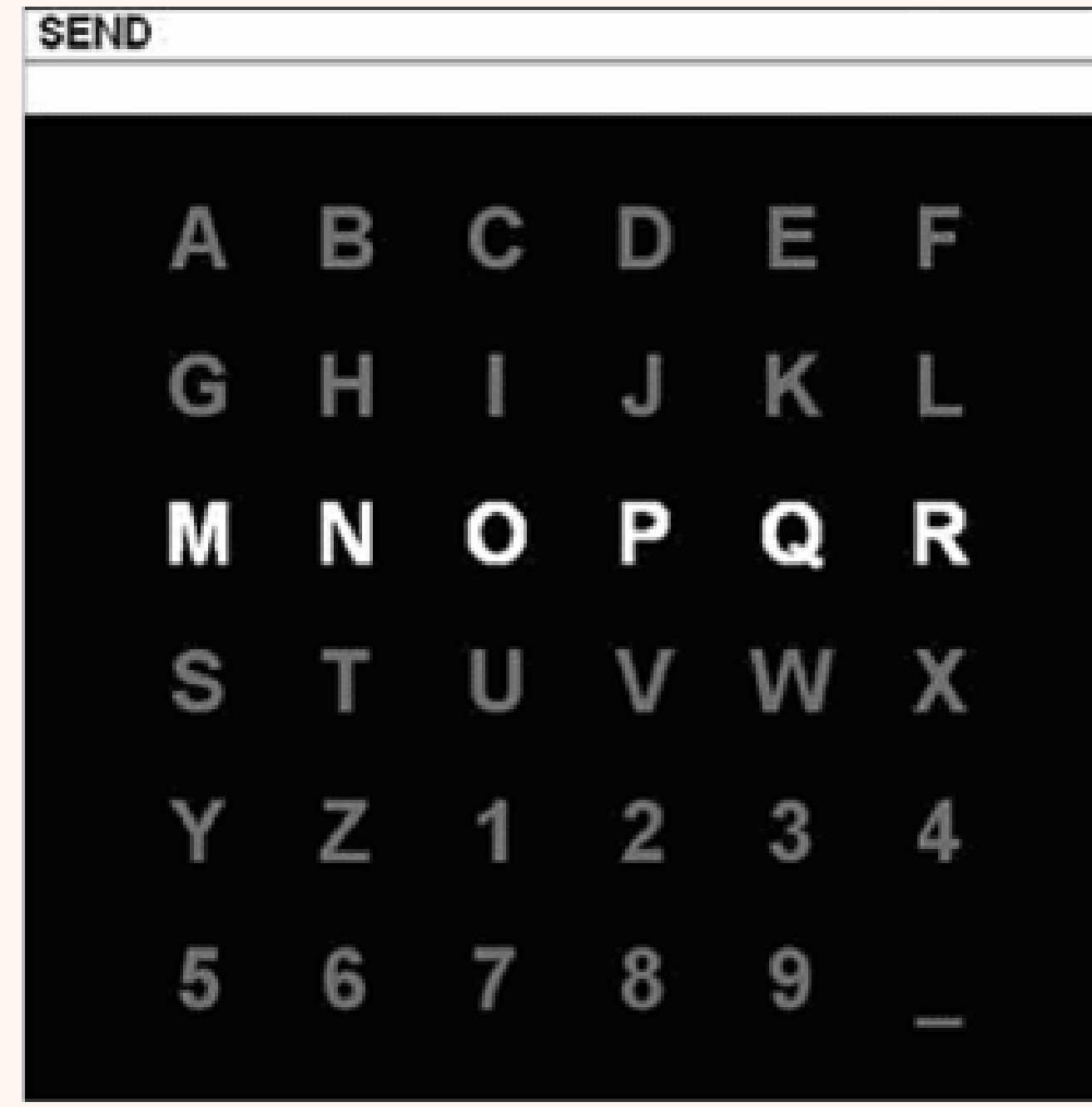
Figure 1. Left to right: A 6 \times 6 matrix used in the P300 speller paradigm, followed by a demonstration of an experiment setup.
